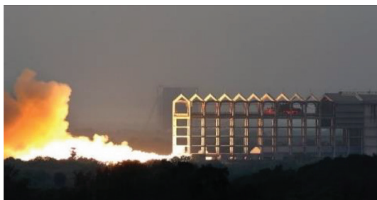
HS200 Static test
