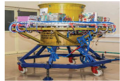
LEA deck with CES avionics
