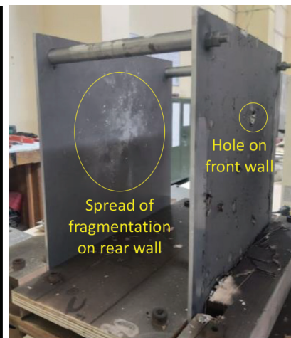
Whipple Shield Test specimen - Post HVI test at 5 km/s
