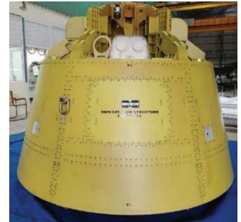
Crew Module sub-assembly for structural test
